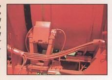
The patented, segmented trommel tube uses bolt-together construction which allows easier replacement of wear parts and many screen attachment options.
