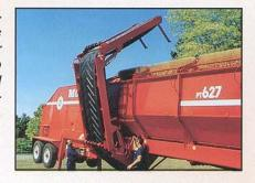
A unique straight through, unrestricted throat opening from hopper to trommel allows the PT737 to accept bulky material. Plugging and jamming is eliminated with a standard anti-plugging device that keeps wet and heavy material from overloading the trommel tube.
