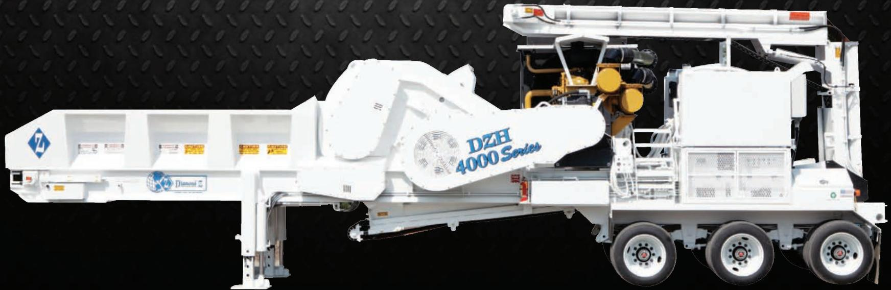
Legendary Diamond Z performance is available in a broad range of horizontal packages. The C18 Caterpillar engine is available in Tier 2, Tier 3, Tier 4i, as well as Tier 4 final. Powerful economical engines, combined with our aggressive down-cut mill, delivers production rates up to 120 tons per hour. The DZH4000 offers easy transportability, friendly operation, ease of maintenance and attention to detail throughout...all hallmark traits of a Diamond Z grinder.
